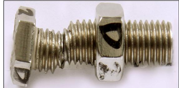
Gambar 12. Tampak samping permukaan geser Baut Stainless Steel Posisi 4.
